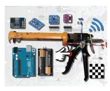
versal" inspection system for soft seals will be developed, which offers high reliability under different environmental conditions. The system is to be designed as a mobile system which is worn on the body in direct human-technology interaction and operated in real time. The execution of the work task is to be evaluated in the process and, if necessary, corrected by appropriate feedback.
